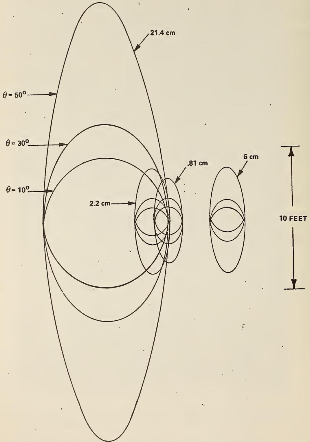
Figure 2.2 Sketch of Radiometer Field-of-View for Various Antenna View Angles (Boom Height = 20 Feet)
